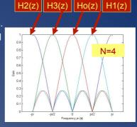
Still, we know this is a PR-FB (see construction previous slides), which means the synthesis filters can apparently restore the aliasing distortion
